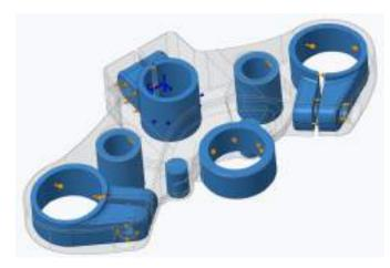
Easily set up optimization by defining the design space, loads and constraint goals, manufacturing process and materials.
