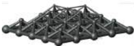
Simplified Representation of Conical Beams in Additive Manufacturing
